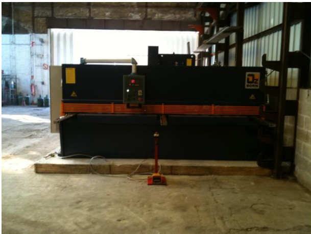
Cisaille Hydraulique 3200X8 mm
