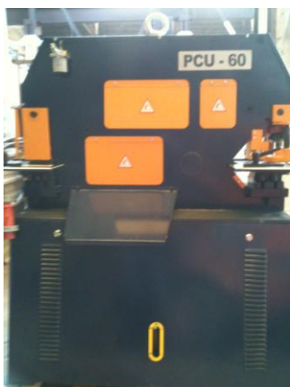
Poinçonneuse Cisaille Universelle 60T
